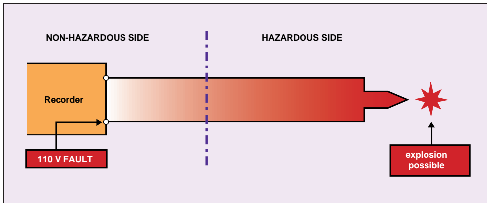
Figure 6. Thermocouple with fault
