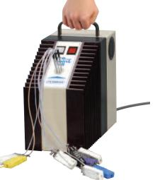
OMEGA's ice point™ is a highly accurate 0°C (32°F) thermoelectric "refrigerator" used in the calibration of temperature instruments. Model TRCIII, \$1175. See page K-12.
