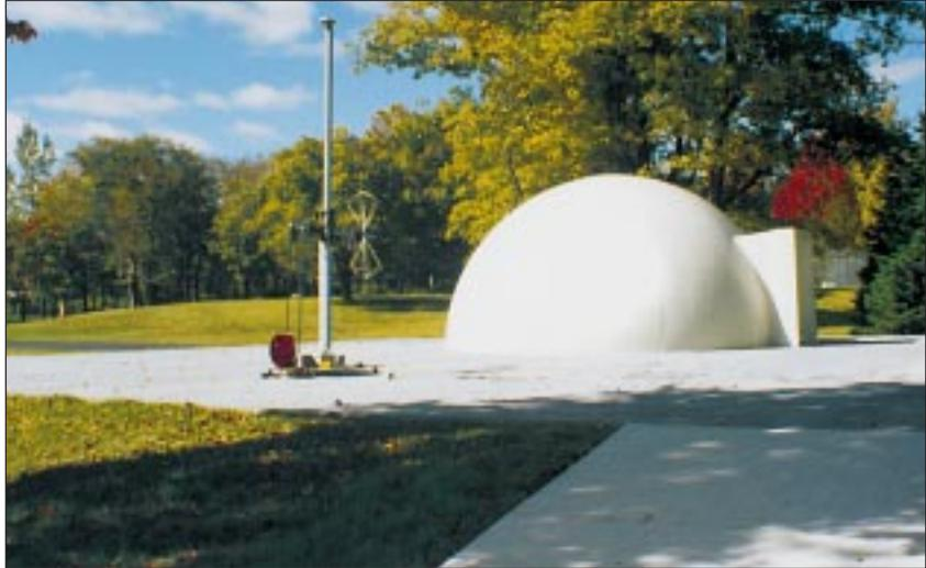
**Open Area Test Site (O.A.T.S.).** Used for 3- and 10-meter testing. It is F.C.C. listed and NVLAP accredited. In addition, the site was assessed by ACEMARK Europe, LTD which is recognized by numerous European competent bodies.
