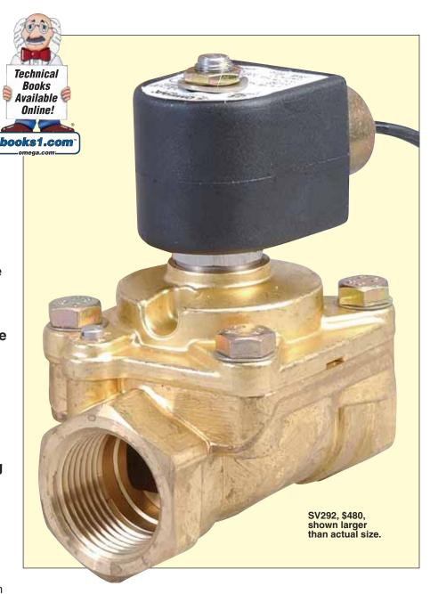
the pilot flow. This is the standard design for the industry. However, to reduce waterhammer in high-flow applications, a unique field adjustment device can effectively control the waterhammer in an application. The closing time on these valves can be adjusted by a 4-position selector. Position 1 allows the fastest closing, position 4 the slowest.
