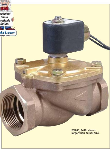
waterhammer in high-flow applications, a unique field adjustment device can effectively control the waterhammer in an application. The closing time on these valves can be adjusted by a 4-position selector. Position 1 allows the fastest closing, position 4 the slowest. There is also a manual override screw that is only used if the coil has failed.
