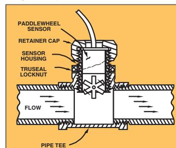
Figure 7: Paddlewheel flow sensor installation and operation
