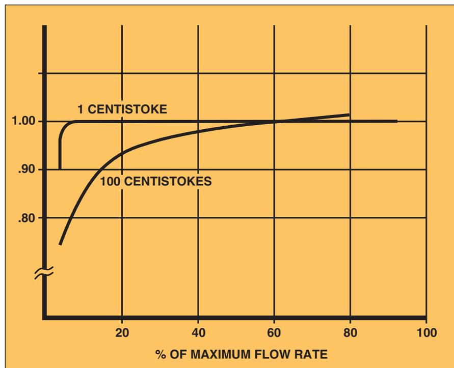
Figure 2: Viscosity effects on a 1" turbine meter
