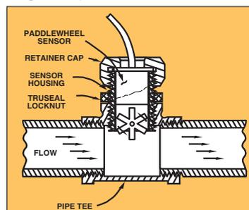
Figure 7: Paddlewheel flow sensor installation and operation
