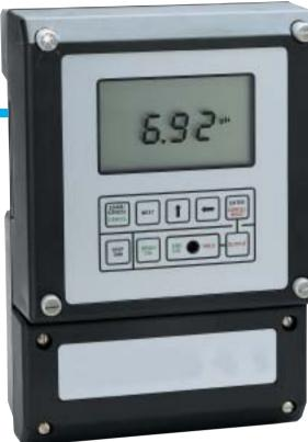
Pressing EXAM/CANCEL changes the display from its measurement mode to an examination mode to show setup variables and their stored values. Pressing the NEXT key displays the next setup variable. The arrow keys change the displayed value to a new value. ENTER stores the displayed value into memory, and EXAM/CANCEL returns the display to its normal measurement mode without changing the stored value.
