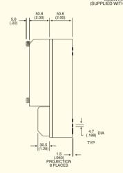
Non-linearity: 0.05% of span Repeatability: 0.1% of span or better TEMPERATURE DRIFT Zero: 0.01% of span per °C Span: 0.01% of span per °C
