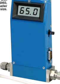
Control Valve: Electromagnetic, normally closed **Output Signal:** Linear 0 to 5 Vdc, 1000  $\Omega$  min load, 4 to 20 mA, 500  $\Omega$  loop resistance Input Power:
