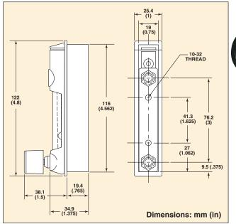
Valve (Optional): Brass or stainless steel cartridge type Seal Material: Buna with brass fittings; FKM with stainless steel
