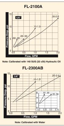
**Pressure Drop:** Approximate pressure losses in flowmeters using oil at normal temperatures. Add 10% to pressure for equal water flows.
