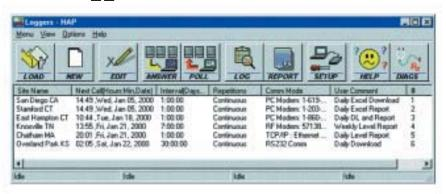
on a PC, the software has a powerful report generation feature that facilitates automatic generation of user designed custom reports. With the report generator, users simply build a report template within Excel. When the logger is interrogated, the template is completed with field data and printed or sent to other applications.
