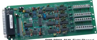
OMB-DBK9, \$549, Eight-Channel RTD Measurement Card, shown smaller than actual size
