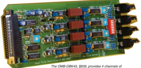
simultaneous sample and hold, as well as low-pass filtering
