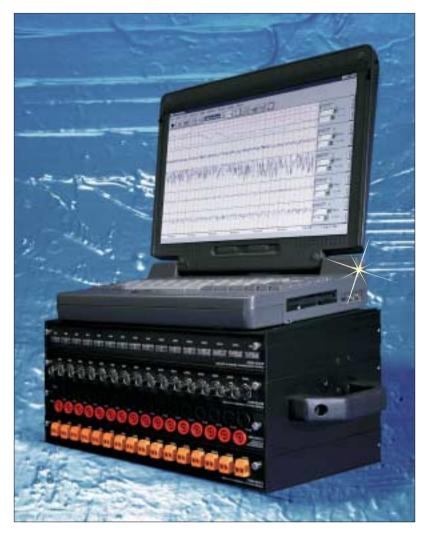
The OMB-CHARTSCAN-1400 portable voltage and temperature recorder is ideal for making isolated temperature and voltage measurements (notebook PC not included)
