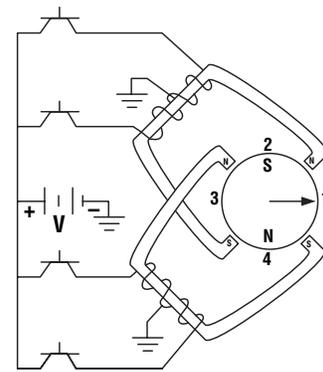
Schematic diagram of a PM motor.
