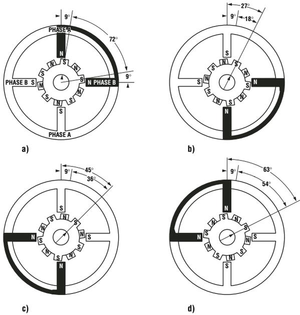
Rotation diagram of 18° Hybrid motor.
