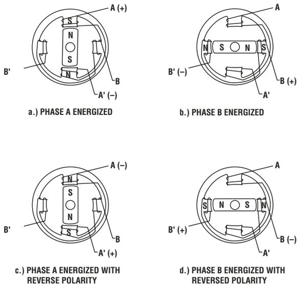
Conventional permanent magnet step motor shown with one phase energized with a bipolar drive. The electromagnetic field rotates in 90° increments. The rotor rotates in 90° increments.
