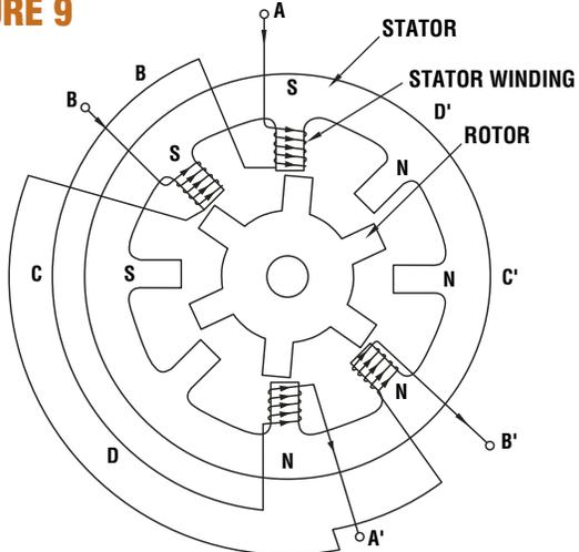
4 phase VR motor with two phases on.
