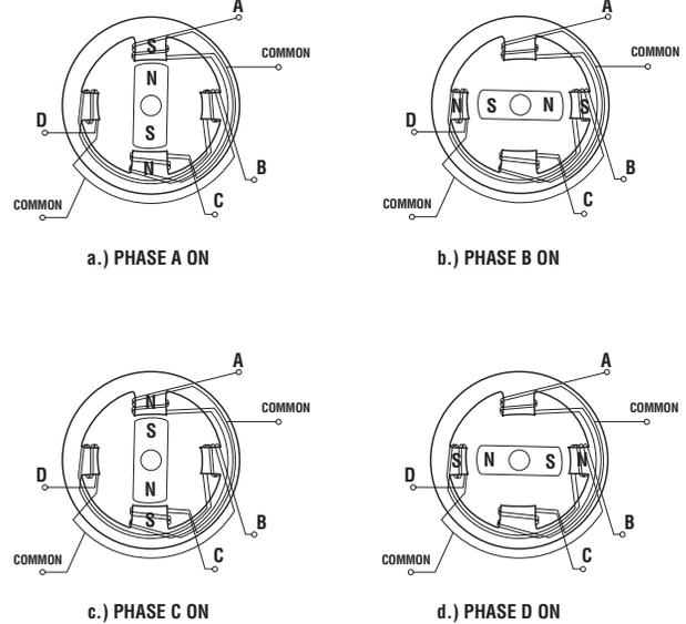
A conventional PM step motor with bifilar winding.
