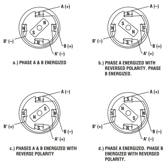
Permanent magnet step motor shown with two phases energized with a bipolar drive.
