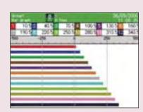
Bar-Graph Screen Display data (measured and virtual) of selected group. Combination display with real-time trend is available.
