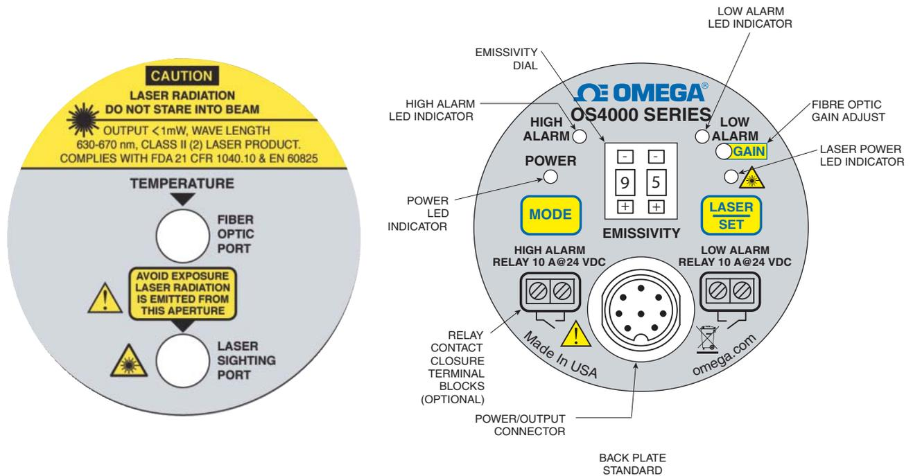
Figure 2 - OS4000 Transmitter Front and Rear Views
