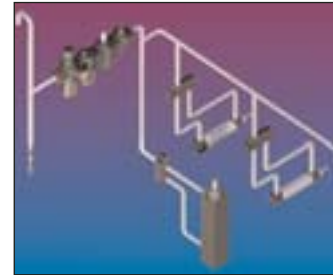
Shut-off valve, filter/reg, micro-fog lubricator, soft start/dump, relief valve.
